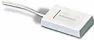
The ASC-SS1 shock sensor protects all types of glass: plate, wired, tempered, and laminated. The sensor will protect the glass within an 8 foot radius from the sensor for glass up to 1/4 inch thick. The ASC-SS1 mounts directly to the glass surface and is wired to a two wire powered protective loop.
